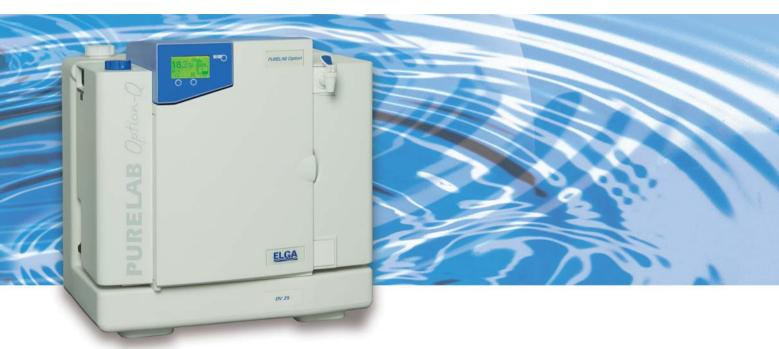
The PURELAB Option-Q is the latest compact ELGA system for producing ultra-pure water without the need for prepurified feed. It can deliver up to 15 liters per hour (100 liters per 8 hour day) of 18.2 M $\Omega$ -cm water\*direct from a potable water supply and dispense this at a flow rate of 1.0 L/min. This makes the PURELAB Option-Q the costeffective choice for many laboratory applications. The PURELAB Option-Q features:
